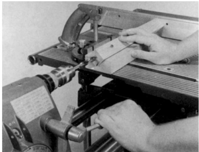
**Figure 11-20.** The V-block can also be used to position a square workpiece for concentric boring.
